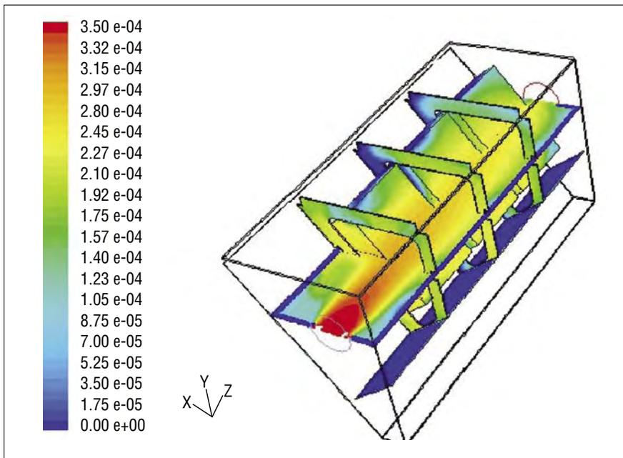
Figure 4. VHP dissemination in the avionics subassembly
