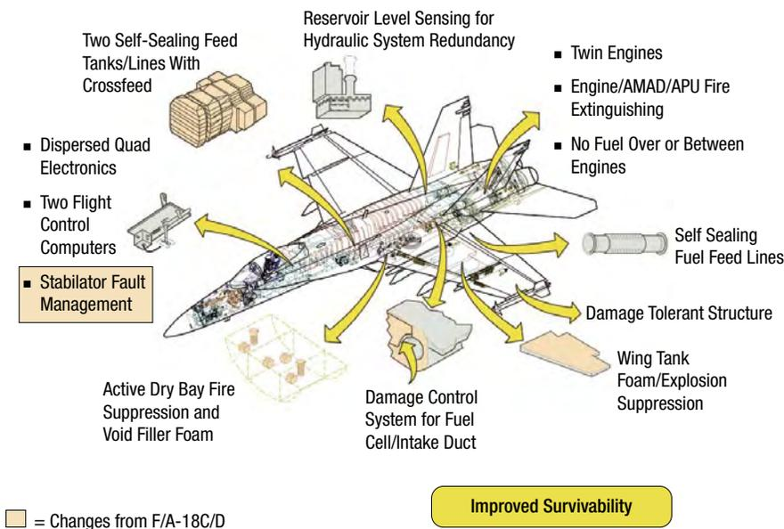
several vulnerability reduction features have also been added to the already rugged design of this C/D variant.
