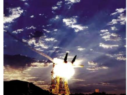
In this F-14 MANPADS test, conducted under the Joint Live Fire program, the objective was to determine the vulnerability of the F-14 to the threat. The aircraft was placed on a platform and was not operating. First-order effects of the threat were determined, as was the method of firing the threat at a stationary target.
