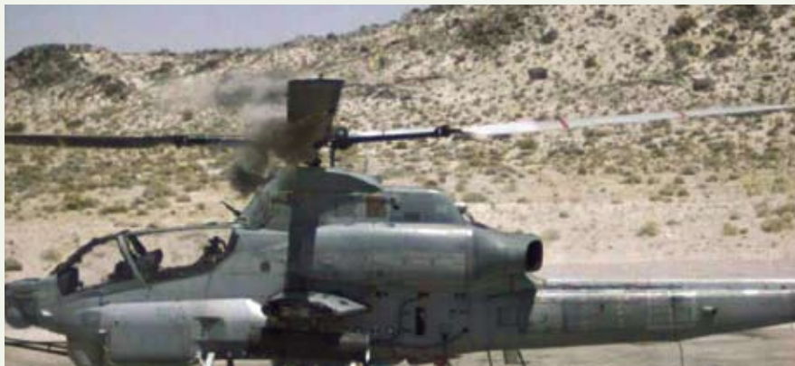
Figure 3. Dynamic main rotor blade test during the AH-1Z FUSL test series.
