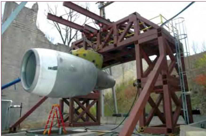
**Figure 2** CF6-50 Engine Mounted on Test Stand
