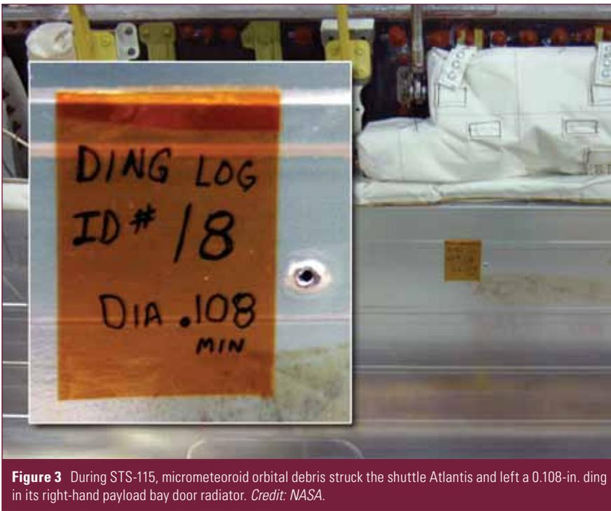
**Figure 3** During STS-115, micrometeoroid orbital debris struck the shuttle Atlantis and left a 0.108-in. ding in its right-hand payload bay door radiator. *Credit: NASA.*
