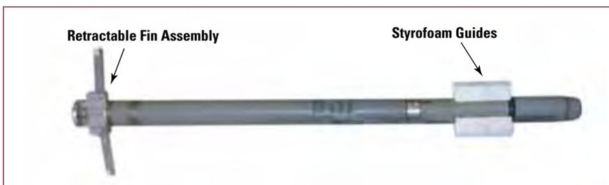
**Figure 1** Example Missile Configuration for Gas-Gun Launch
