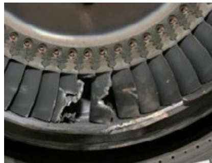
Figure 3 Damage to the Gas Generator Turbine Rotor
