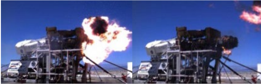
Figure 6 Fuel Leak and Fire with Self-Extinguish
