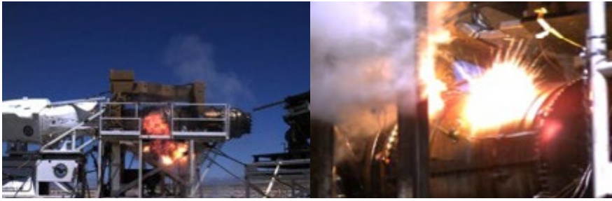
Figure 5 F135 Ballistic Test Events (Fuel System Component and Fan Case)
