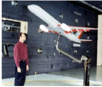
Figure 5 Generic Transport Aircraft Model in the NASA 14x22 Wind Tunnel
