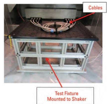
**Figure 3** Test Fixture Mounted to Shaker in Chamber
