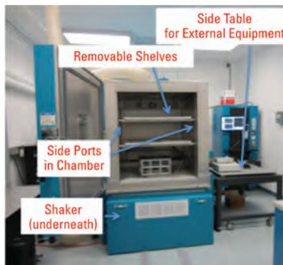
**Figure 2** Government Thermal/Vibration System with Side Tables for External Equipment
