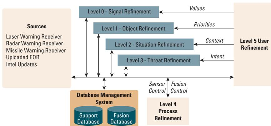
Figure 4 Fusion Inputs/Outputs [4]
