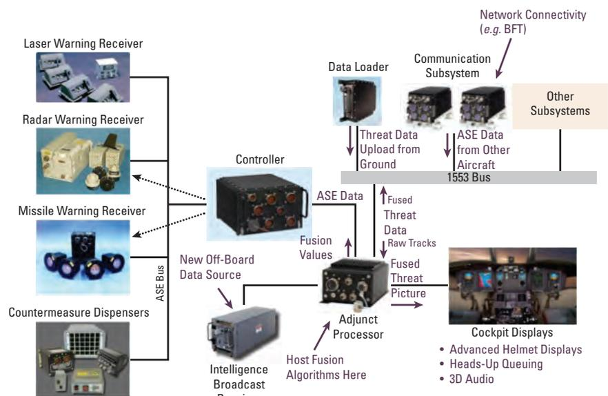
**Figure 3** Onboard/Offboard IASE [3]
