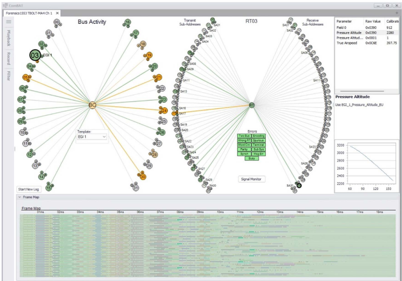
Figure 3. Typical MIL-STD-1553b Data Bus Traffic.
